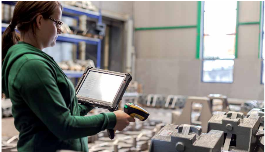
Figure 3: The new mobile dispatch management system implemented at Casper clearly identifies each packed and barcode labelled casting during loading
