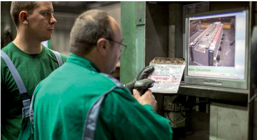
Figure 2: The system displays information on the current manufacturing status and instructions at the start of every new job
